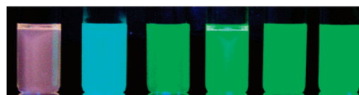
Figure 3. UV-vis absorption and PL spectra (top) of the “nano-onions” with CdSe cores capped alternately by CdS and CdSe shells, and the corresponding luminescence image (bottom) for the samples under UV lamp irradiation.
